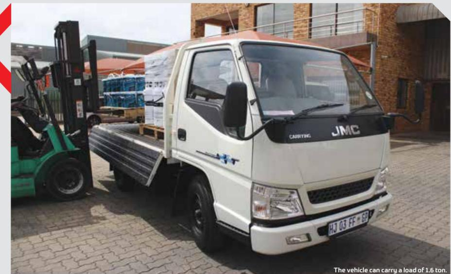
The vehicle can carry a load of 1.6 ton.
